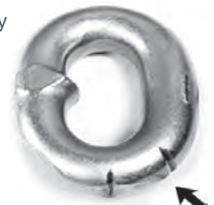
Figure 2: Location of nicks, gouges, and notches will dictate their severity.
